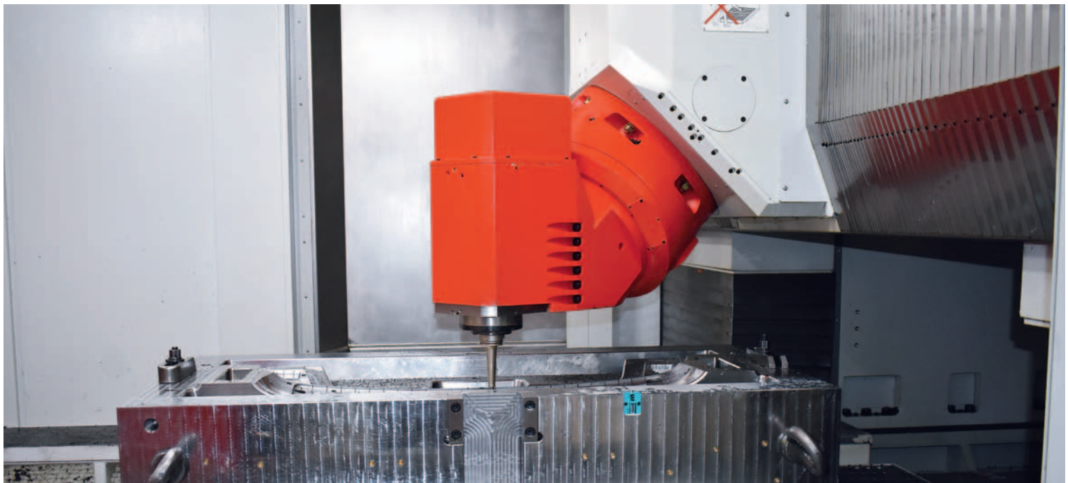
5-axis machining of an injection-mould
