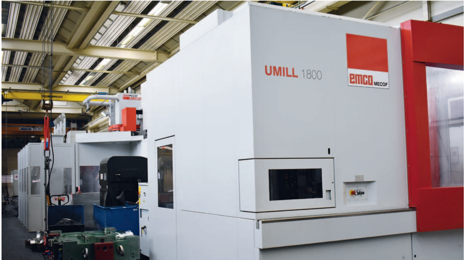
Gantry type 5-axis milling and turning centre Umill 1800 in operation at HKR in Spraitbach, manufacturer of high-precision injection mould tools
