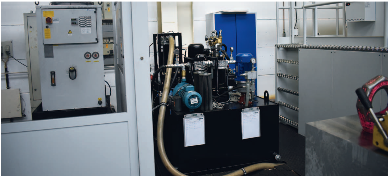
Combined coolant system, which is used both for the ECOMILL as well as the UMILL 1800
